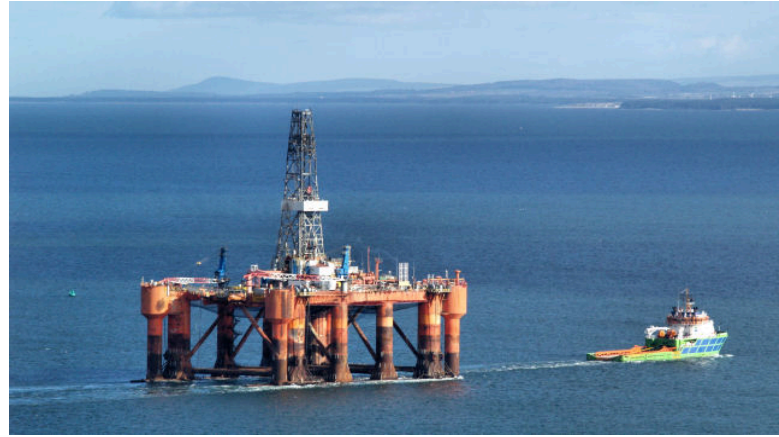
FIGURE 8 OILRIG BEING TOWED TO SITE OF OIL EXTRACTION
